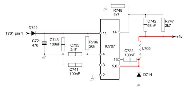
This DC-DC converter will operate from a supply between 8v to 55v and produces an output voltage of between 3v3 and 50v depending on the value of R747 (5v output R747 = 2k7). C741 connected to pin 3 provides a soft-start routine. If pin 3 is held low then the device will not operate. The frequency of the internal oscillator is fixed by the value of R706 and C735. Over-current and over-voltage protection is incorporated into the design of this device.
