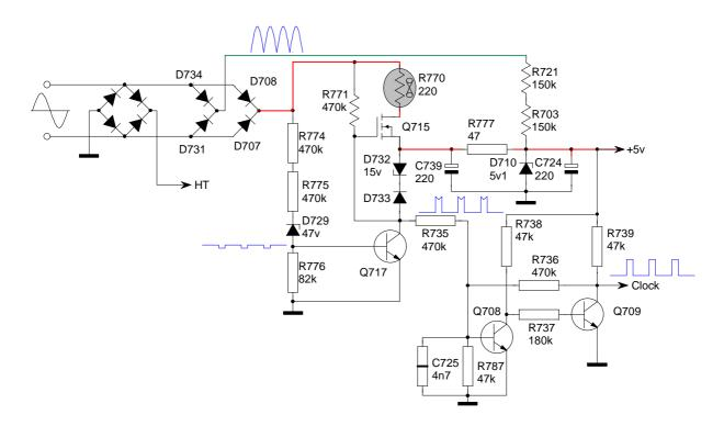
When Q717 turns on the gate of Q715 is taken to ground. Since this is a N Channel MOSFET Q715 is turned off and no current will flow through this device.
