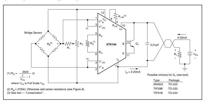
FIGURE 1. Bridge Sensor Application, Connected for Positive Nonlinearity.
