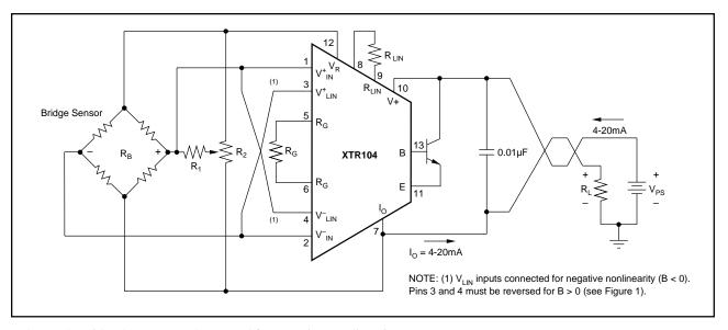
FIGURE 3. Bridge Sensor,  $V_{\text{LIN}}$  Connected for Negative Nonlinearity.
