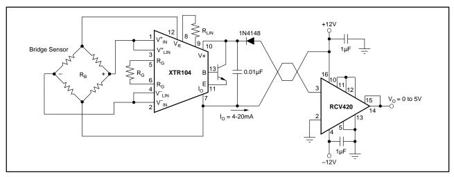
FIGURE 9. ±12V-Powered Transmitter/Receiver Loop.
