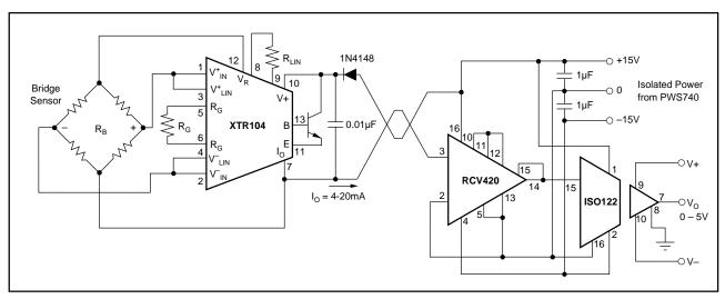
FIGURE 10. Isolated Transmitter/Receiver Loop.
