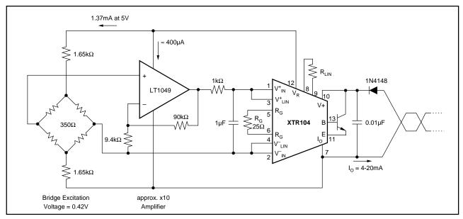
FIGURE 8.  $350\Omega$  Bridge With X10 Preamplifier.
