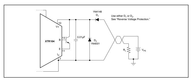
FIGURE 6. Reverse Voltage Protection.
