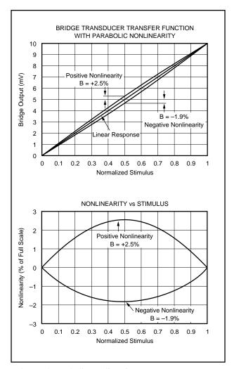
FIGURE 4. Parabolic Nonlinearity.
