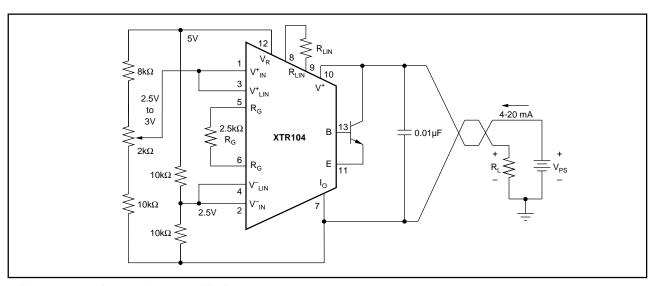
FIGURE 5. Potentiometer Sensor Application.
