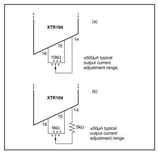
FIGURE 2. Low-scale Output Current Adjustment.
