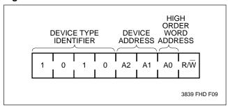
The next two significant bits address a particular device. A system could have up to four X24C04 devices on the bus (see Figure 10). The four addresses are defined by the state of the  $A_1$  and  $A_2$  inputs.
