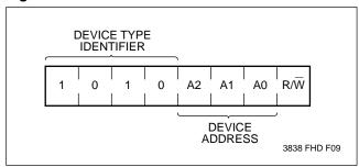
The next three significant bits address a particular device. A system could have up to eight X24C02 devices on the bus (see Figure 10). The eight addresses are defined by the state of the  $A_0$ ,  $A_1$  and  $A_2$  inputs.
