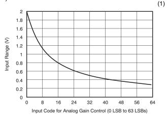
Figure 12. Analog Gain vs Setting Code
