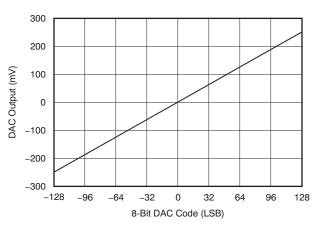
Figure 15. Offset DAC Setting Code vs Output Voltage
