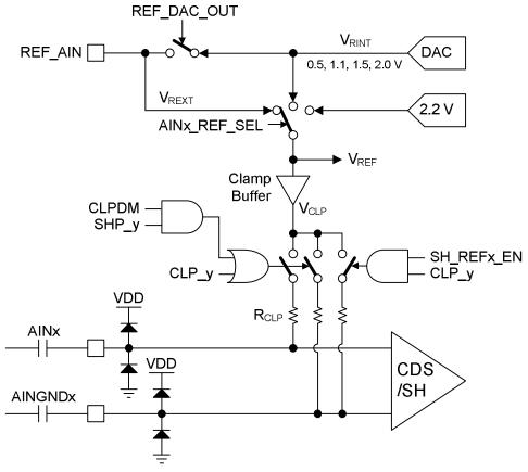
(1) If the sensor signal is directly input to the AFE, the enternal capacitor should not be connected.
