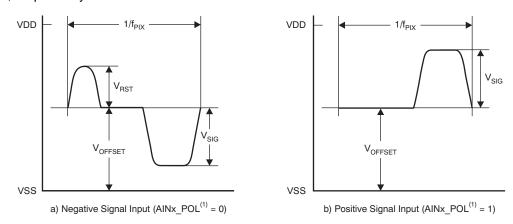
Figure 1. Analog Input Definition
