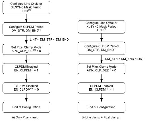
(1) Internal registers: AINx\_CLP\_SEL = addresses 16 and 17; LINT = address 7; DM\_STR = address 8; DM\_END = address 9; and EN\_CLPDM = address 399, bit 1.
