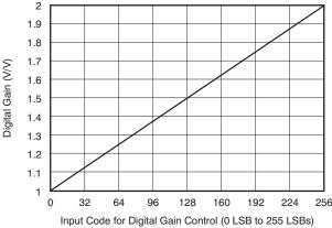
Figure 14. Digital Gain Setting Code
