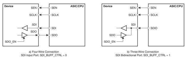
Figure 23. SPI Connection Between AFE and System
