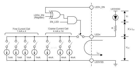
Figure 20. LED Driver Block Diagram
