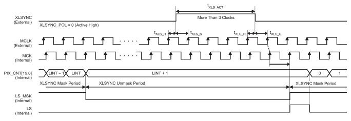
Figure 17. External Line Synchronous Mode (XLSYNC\_SEL = 0, default)
