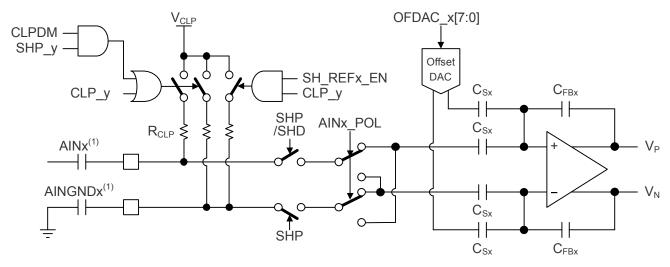
Figure 4. CDS Mode Input Circuit for CCD Signal
