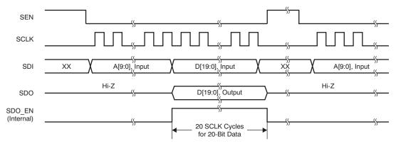
Figure 24. SPI Signal Flow of Read Mode for Four-Wire Connection
