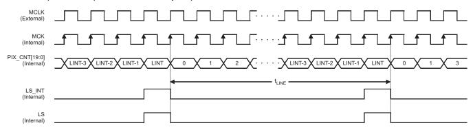
Figure 16. Internal Line Synchronous Mode (XLSYNC\_SEL = 1)
