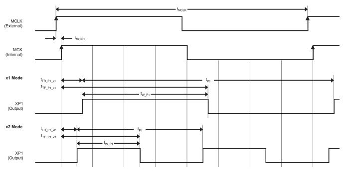
Figure 19. XP1 Fast Transfer Clock Pulse Setting
