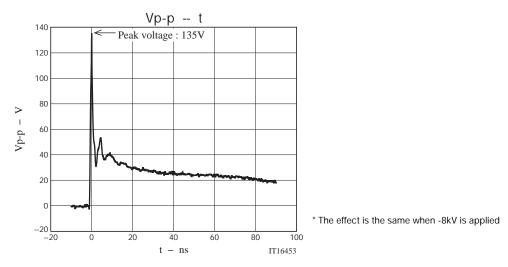
IEC61000-4-2 Contact Disdharge, when 8kV is applied
