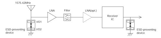
Either I/O1 or I/O2 can be connected to GND (the same performance)
