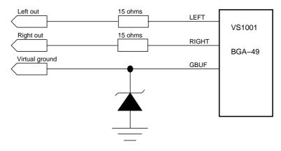
Figure 21: ESD Protection for BGA-49 Package.
