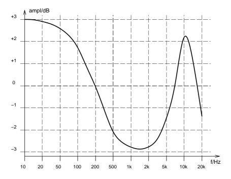
Figure 11: Built-In Bass/Treble Enhancer Frequency Response at 44.1 kHz.
