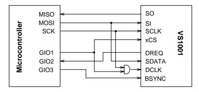
Figure 13: 6-Pin VS1001k Connection.
