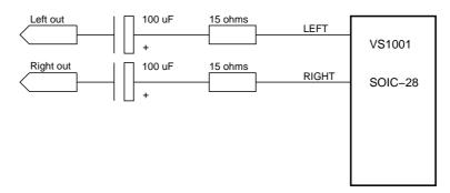
Figure 20: ESD Protection for SOIC-28 Package.
