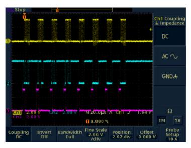
Figure 15: Oscilloscope Picture: Sending Eight SDI Bytes.
