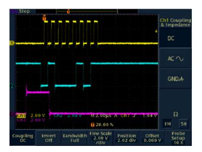
Figure 14: Oscilloscope Picture: Sending One SDI Byte.
