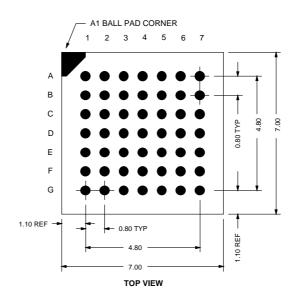
Figure 2: Pin Configuration, BGA-49.
