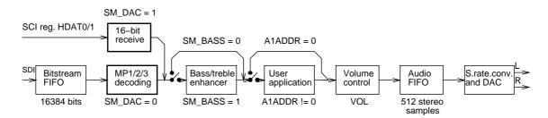
Figure 10: Data Flow of VS1001k.
