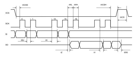
Figure 9: SPI Timing Diagram.
