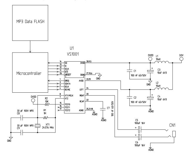
Figure 4: Typical Connection Diagram Using SOIC-28.
