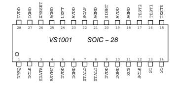
Figure 1: Pin Configuration, SOIC-28.
