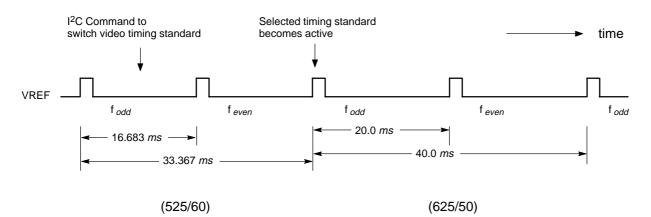
Fig. 3–4: Transition between timing standards
