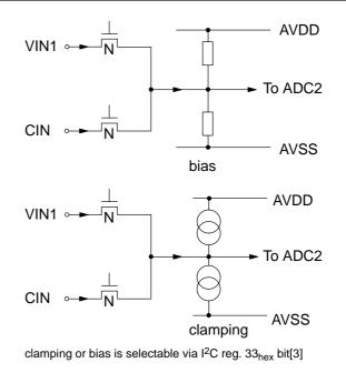
Fig. 6-14: Video Inputs ADC2
