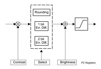
Fig. 2–18: Contrast and brightness adjustment
