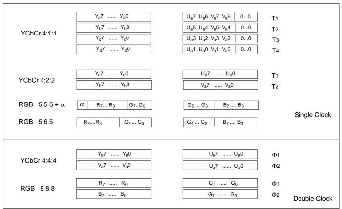
Fig. 2–22: Byte formats for double port transfers
