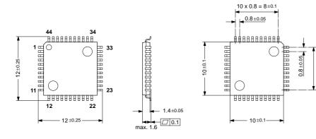
**Fig. 6–2:** 44-Pin Plastic Thin-Quad-Flat-Pack **(PTQFP44F)** Weight approximately 0.35 g Dimensions in mm
