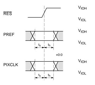
**Fig. 6–17:** I<sup>2</sup>C Selection: Slave Address (PREF) and Init Table (PIXCLK)
