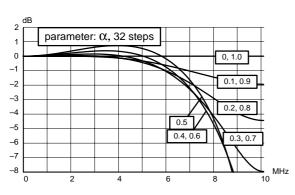
Fig. 2–14: Luminance skew filter magnitude frequency response
