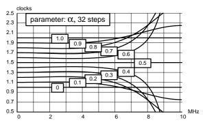
Fig. 2–15: Luminance skew filter group delay characteristics
