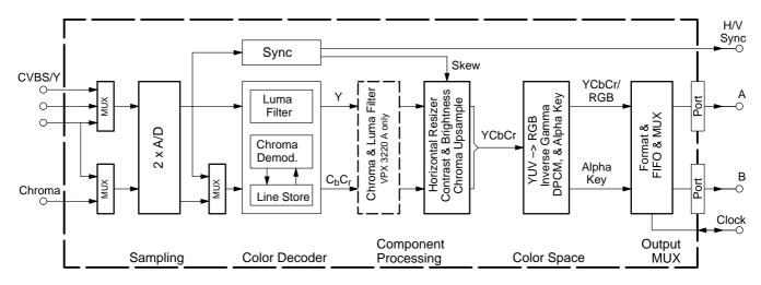
Fig. 1–1: Block diagram of the VPX
