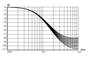
**Fig. 2–5:** Frequency response of SECAM deemphasis
