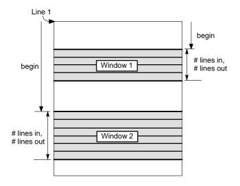
Fig. 3-6: Vertical dimensions of windows
