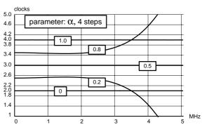
Fig. 2–17: Chrominance skew filter group delay characteristics
