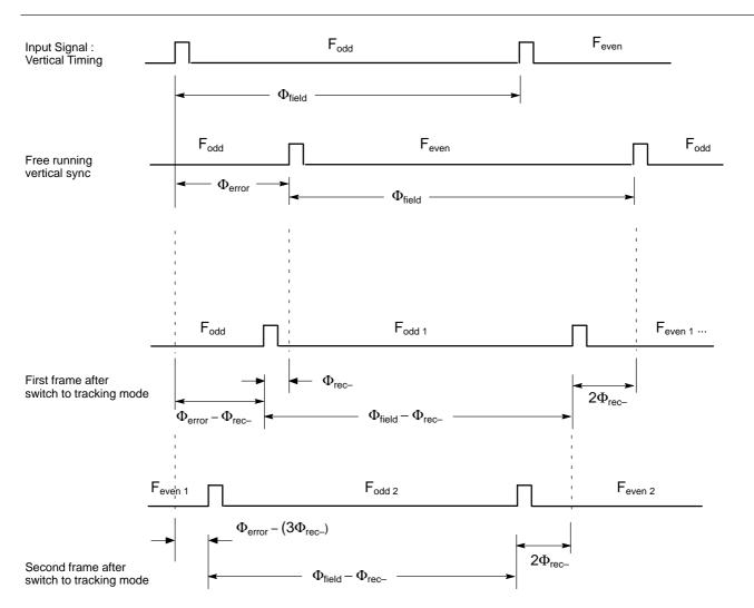
Fig. 3–5: Synchronization to analog input
