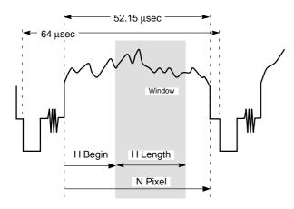
Fig. 3-9: Horizontal Dimensions of Sampling Window
