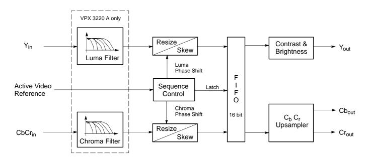
Fig. 2-10: Component processing stage
