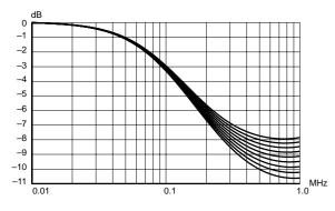
**Fig. 2–7:** Frequency response of SECAM deemphasis
