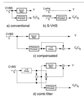
Fig. 2–8: NTSC color decoding options
