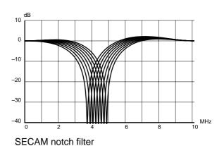
Fig. 2–11: Frequency responses of the luma notch filter for PAL, NTSC, SECAM
