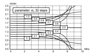
**Fig. 2–13:** Luminance, chrominance skew filter group delay characteristics
