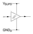
Fig. 4-3: Input pins RESQ, TEST
