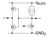
Fig. 4-6: Input/Output pins PR0-PR2, FPDAT
