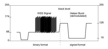
Fig. 2–15: PAL+ helper reference line output signal
