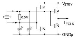
Fig. 4-8: Input/Output Pins XTAL1, XTAL2
