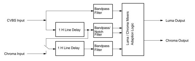
Fig. 2-3: Block diagram of the adaptive comb filter
