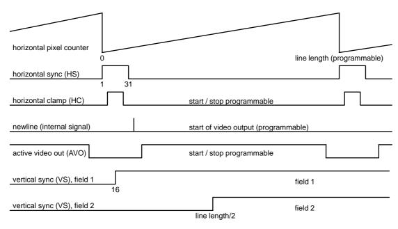
Fig. 2–14: Horizontal timing for line-locked mode
