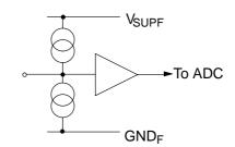
Fig. 4–12: Input pins VIN1–VIN3
