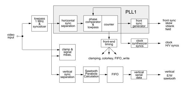
Fig. 2-16: Sync separation block diagram
