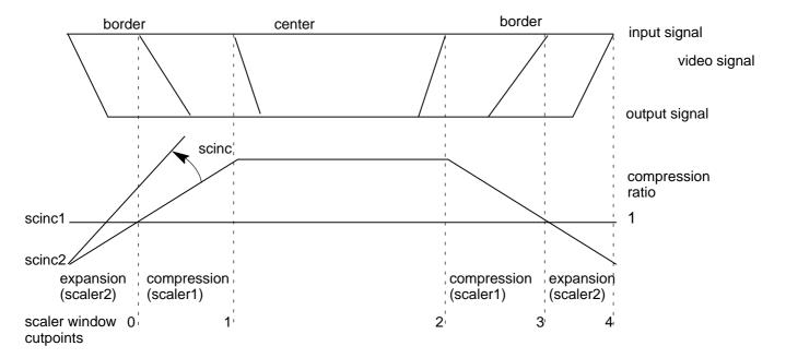
Fig. 3–2: Scaler operation for "panorama" mode at 13.5 MHz
