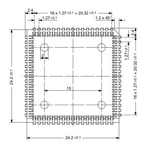
Fig. 4–1: 68-Pin Plastic Leaded Chip Carrier Package (PLCC68) Weight approximately 4.8 g Dimensions in mm
