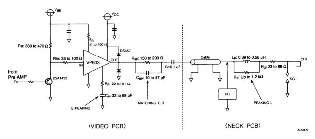
Mounting location for the C, G matching circuit Add the RC matching circuit at a position as close as possible to the VP603 output pin.
