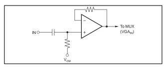
Figure 58. Recommended Circuit for Coupling an External Signal into the MUX
