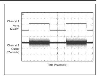
Figure 64. Response to Step Change of V<sub>CNTL</sub>
