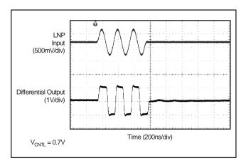
Figure 70. Extreme Overload (2V<sub>PP</sub> Input)
