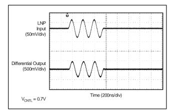
Figure 67. Before Overload (100mV<sub>PP</sub> Input)
