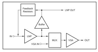
Figure 56. Block Diagram of LNP/VGA Interface
