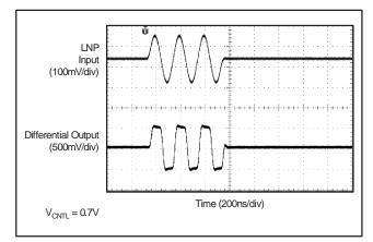
Figure 69. Overload (240mV<sub>PP</sub> Input)
