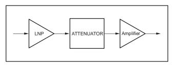
Figure 54. Block Diagram of Older VCA Models
