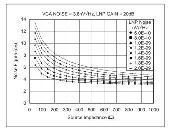
Figure 62. Noise Figure for Conventional Termination
