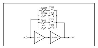
Figure 59. Feedback Resistor Network
