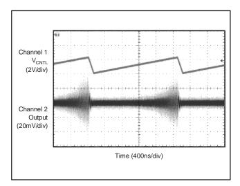
Figure 65. Response to Ramp Change of V<sub>CNTL</sub>
