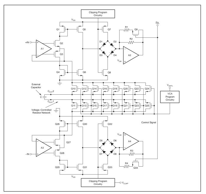
Figure 63. Block Diagram of VCA
