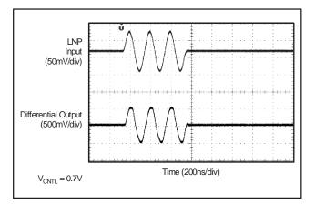
Figure 68. Approaching Overload (120mV<sub>PP</sub> Input)
