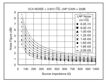
Figure 61. Noise Figure for Active Termination
