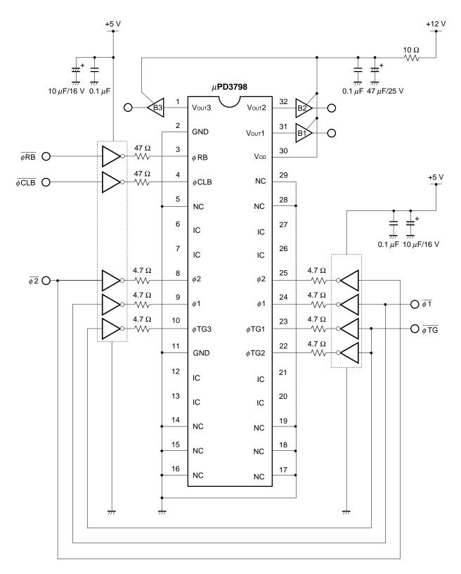
Cautions 1. Leave pins 6, 7, 12, 13, 20, 21, 26, 27 (IC) unconnected. 2. Connect the No connection pins (NC) to GND.
