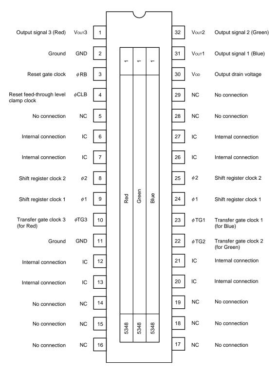
Cautions 1. Leave pins 6, 7, 12, 13, 20, 21, 26, 27 (IC) unconnected. 2. Connect the No connection pins (NC) to GND.
