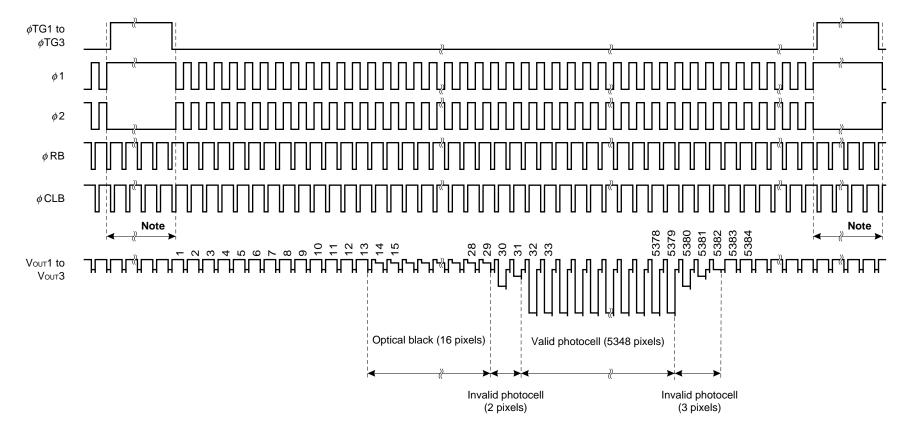
**Note** Input the  $\phi$ RB and  $\phi$ CLB pulses continuously during this period, too.
