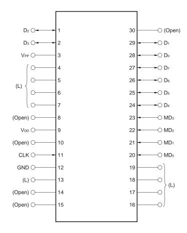
CautionContents in parantheses indicate how to handle unused pins in PROM programming mode.L:Connect to GND via a resistor (470 Ω) separately.OPEN:Leave unconnected.
