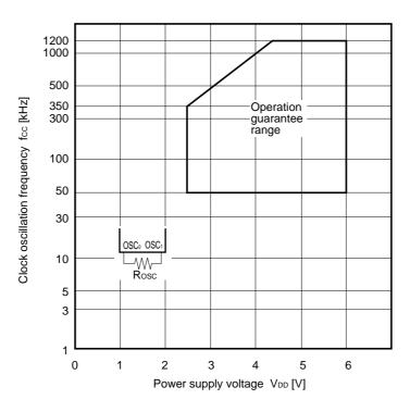
Rosc vs.  $V_{DD}$  for Operation Guarantee Range (T<sub>A</sub> = -40 to +85 °C)
