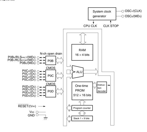
**Remark** Pin names enclosed in parentheses are used in PROM programming mode.
