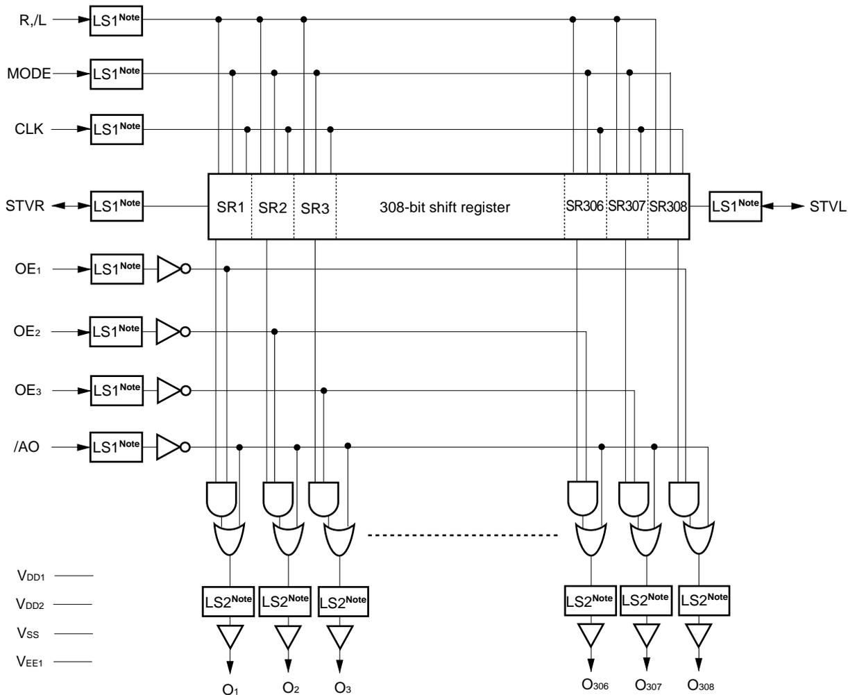
**Note** LS1: shifts CMOS level and internal level, LS2: shifts interval level and output level ( $V_{DD2}$  to  $V_{EE1}$ ).
