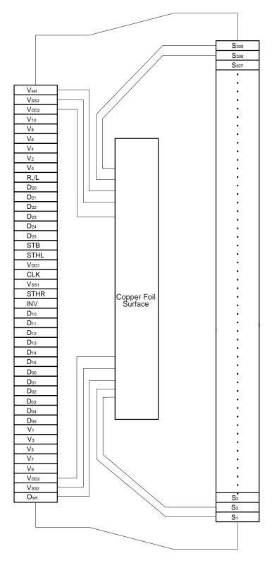
$\label{eq:result} \textbf{Remark} \ \ O_{sel} \ and \ V_{sel} \ pins \ are \ internally \ pulled \ up.$
