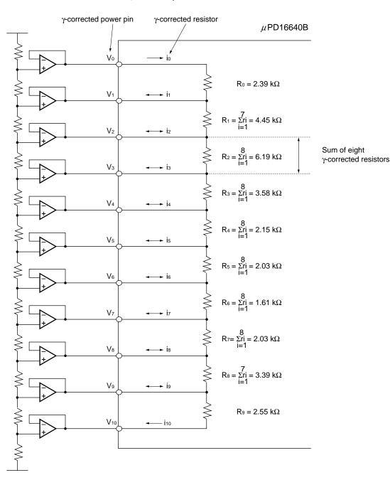
Figure4–2. γ-Corrected Power Circuit
