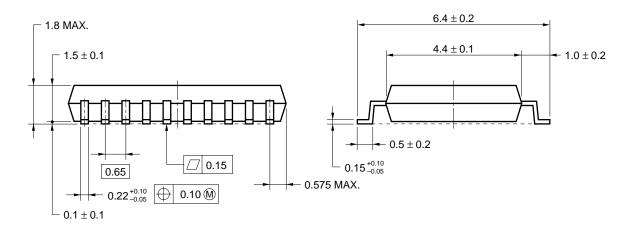
**NOTE** Each lead centerline is located within 0.10 mm of its true position (T.P.) at maximum material condition.
