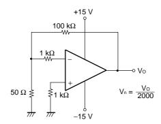
Figure 2 Channel Separation Measurement Circuit
