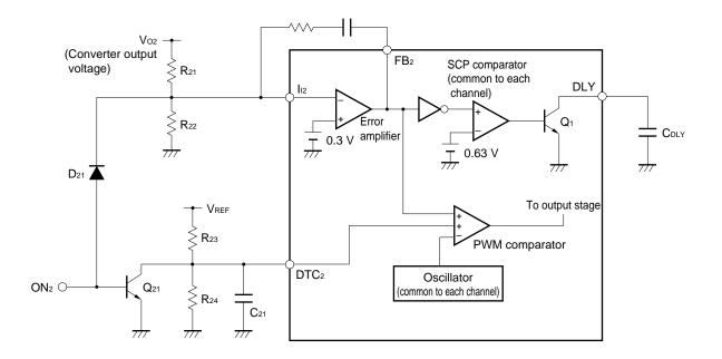
The sequence in which channel 2 is turned ON/OFF is as follows:
