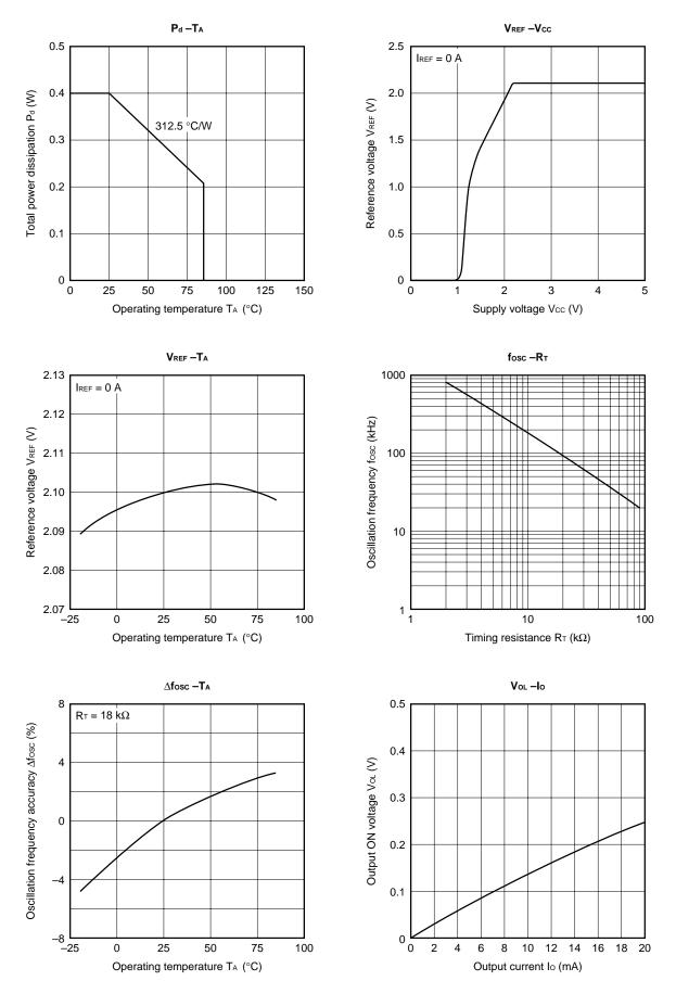
TYPICAL CHARACTERISTIC CURVES (Unless otherwise specified, Vcc = 3 V, fosc = 100 kHz, TA = 25 °C)
