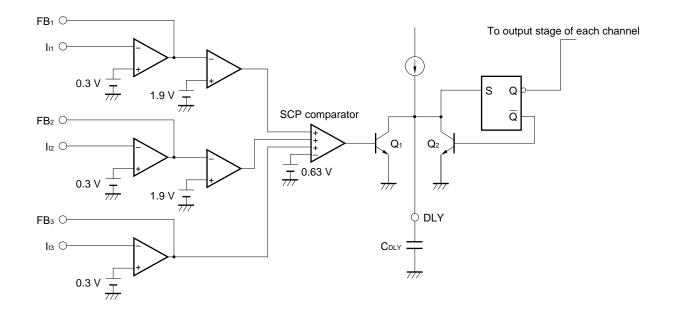
The timer latch circuit operates as follows:
