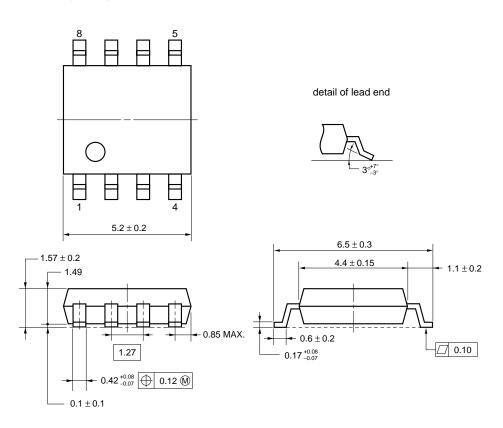
**NOTE** Each lead centerline is located within 0.12 mm of its true position (T.P.) at maximum material condition. See connection diagram for description of leads.
