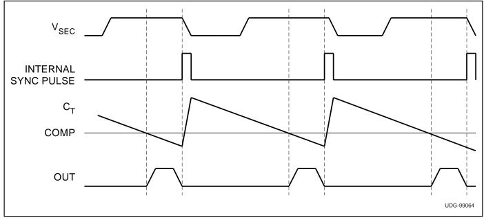
Figure 1. Trailing edge synchronization, leading edge modulation.
