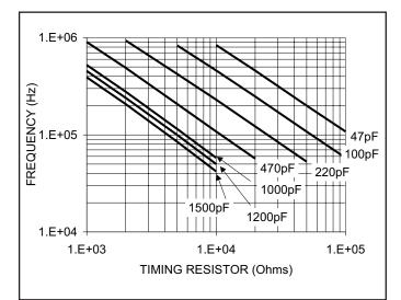
Figure 2. Oscillator frequency vs.  $R_T$  with  $C_T$  as a parameter.
