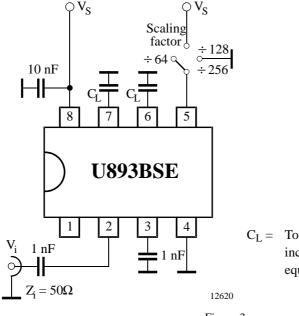
$$\begin{split} C_L = & \quad \text{Total capacitive output load} \\ & \quad \text{including test fixture and test} \\ & \quad \text{equipment capacitance} \end{split}$$
