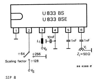
$L_1 = L_2 = 150 \text{ nH (6 turns CuL 0.45 mm Ø on 4 mm Ø)}$
