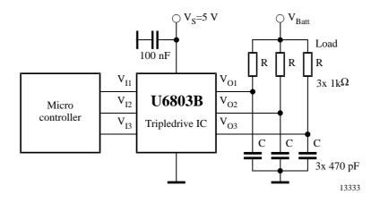
Figure 3. Application schematic
