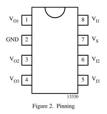
Integrated circuit, U6803B, requires a stabilized supply voltage (V<sub>S</sub> = 5 V±5%) to comply with its electrical characteristics. An external buffer capacitor of C = 100 nF value is recommended. An integrated 14-V Zener-diode between V<sub>S</sub> and ground protects the supply pin.
