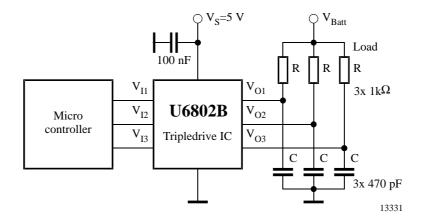
Figure 3. Application schematic
