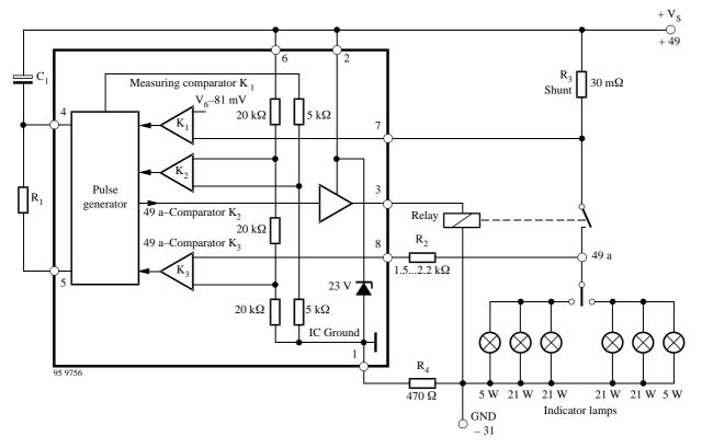
$\begin{array}{c} Figure \ 1. \ Application \ circuit \ as \ a \ car \ flasher \\ Resistor \ R_1, \ R_2 \ and \ R_4: \ 1/4 \ Watt \\ R_4 \ for \ protection \ against \ continuous \ reversed \ polarity: 0.5 \ Watt \end{array}$
