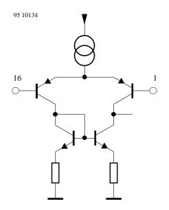
Figure 19. Pin 16 OP<sub>in-</sub>
