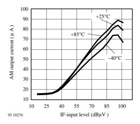
Figure 25. AM-demodulator characteristic vs. temperature
