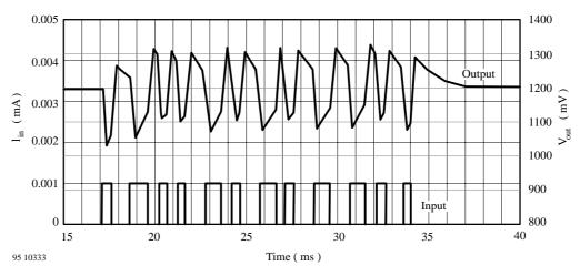
Figure 20. Time domain response of 2-kHz Bessel lowpass data filter
