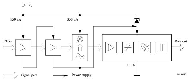
Figure 29. Principle diagram of a UHF remote control receiver
