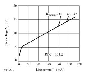
Figure 5. Typical DC characteristics for various SWAMP resistors
