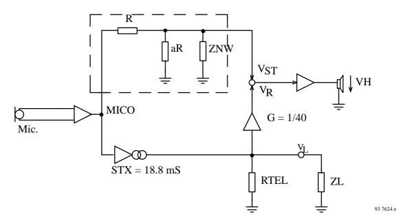
Figure 7. Schematic of the side tone
