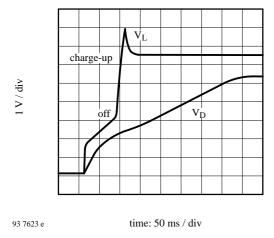
Figure 6. Charge up characteristics at  $I_L = 20 \text{ mA}$
