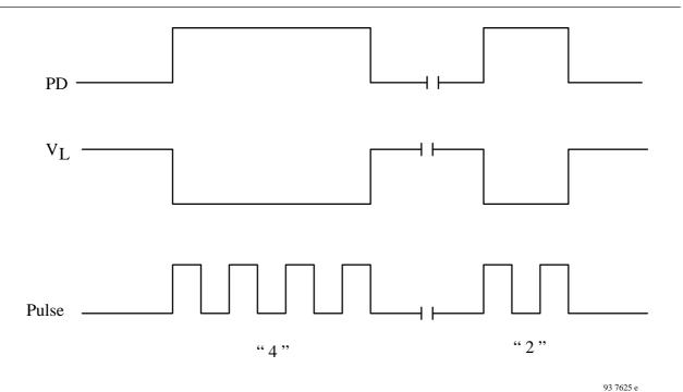
Figure 8. Recommended timing diagram for power down diagram
