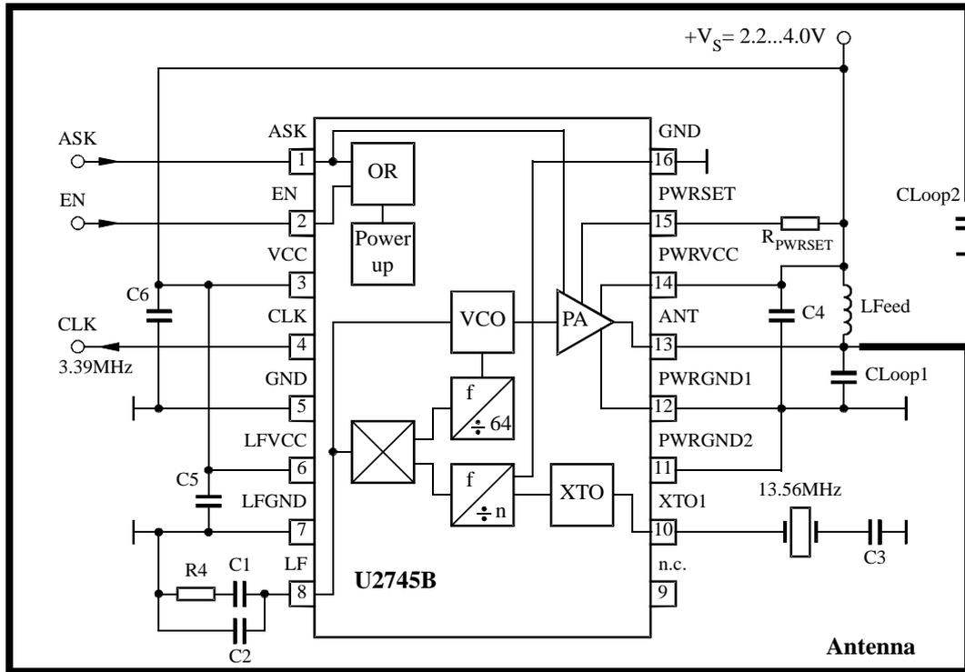
Figure 5. Application circuit
