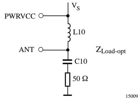
Figure 4. Measurement output network
