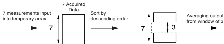
Figure 28. MAV Filter Operation (Patent Pending)
