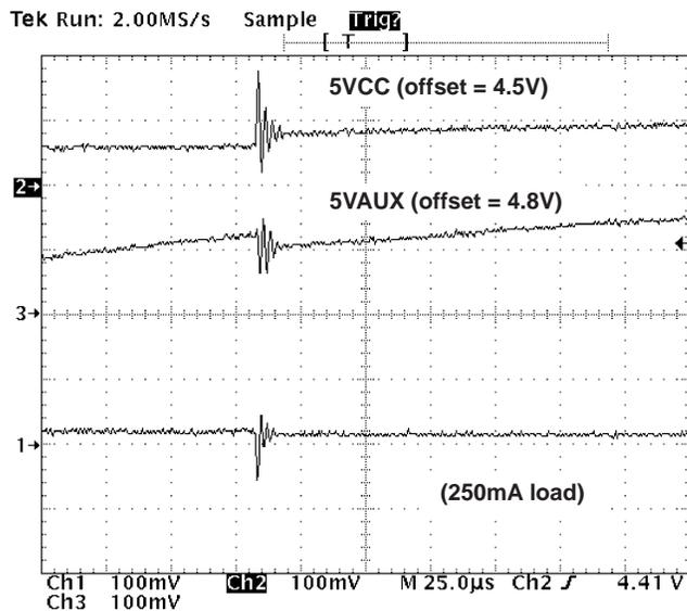
Figure 3. 5VCC Power Up (5VAUX = 5 V)
