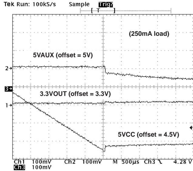
Figure 7. 5VCC Power Down (5VAUX = 5 V)
