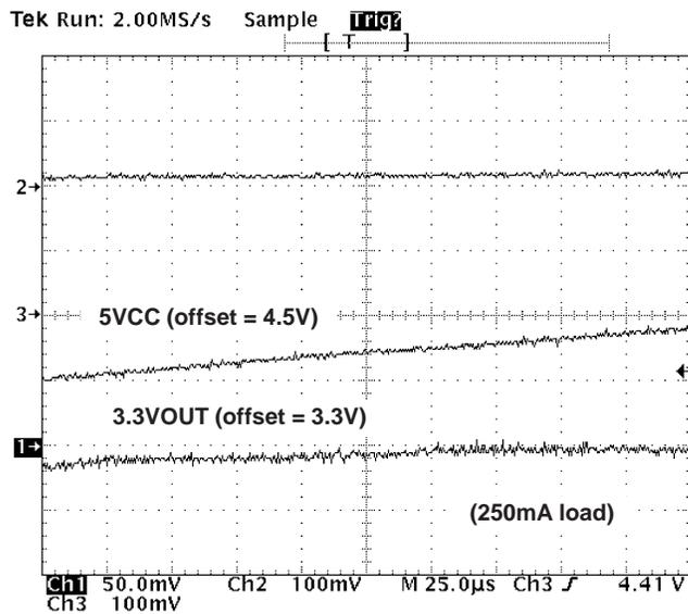
Figure 4. 5VCC Power Up (3.3VAUX = 3.3 V)
