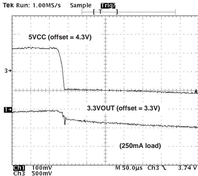
Figure 6. 5VCC Power Down (3.3VAUX = 3.3 V)
