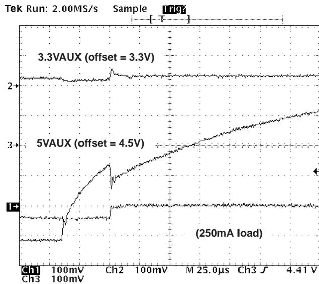
Figure 5. 5VAUX Power Up (3.3VAUX = 3.3 V)
