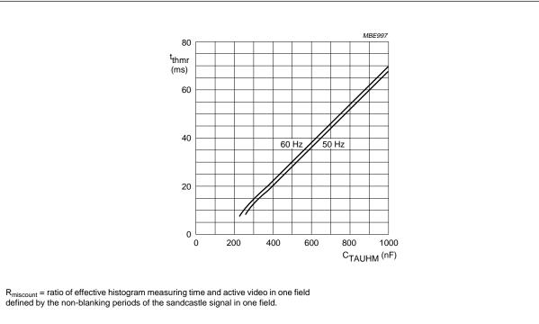
Fig.3 Response speed of average histogram amplitude control loop as a function of  $C_{TAUHM}$  at both 50 and 60 Hz field rate ( $R_{miscount} = 1$ ;  $C_{HMx} = 10$  nF).
