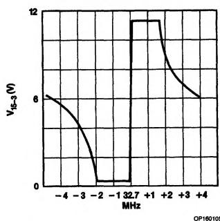
Figure 1. AFC Output Voltage  $V_{15-3}$  for Positive AFC
