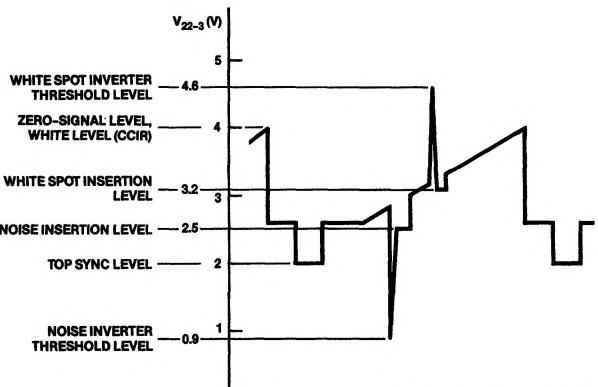
Figure 3. Video Output Waveform Showing White Spot and Noise Inverter Threshold Levels
