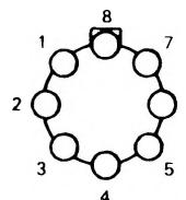
Pin 4 connected to case
