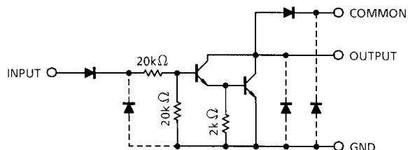
Note: The input and output parasitic diodes cannot be used as clamp diodes.
