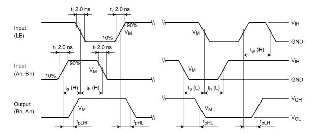
Figure 4  $t_{pLH}$ ,  $t_{pHL}$ ,  $t_{w}$ ,  $t_{s}$ ,  $t_{h}$
