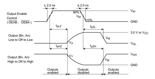
$\textbf{Figure 6} \quad t_{pLZ},\, t_{pHZ},\, t_{pZL},\, t_{pZH}$
