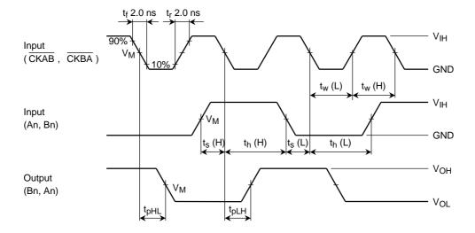
Figure 3  $t_{pLH}, t_{pHL}, t_w, t_s, t_h$
