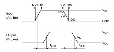
Figure 2 t<sub>pLH</sub>, t<sub>pHL</sub>
