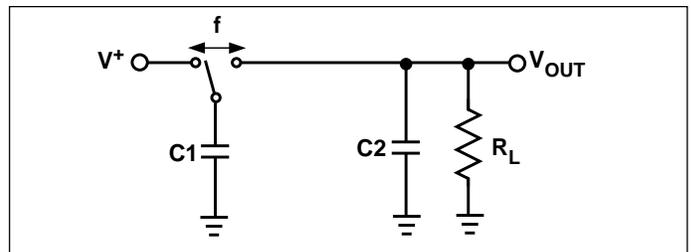
Figure 2a. Ideal Switched Capacitor Model
