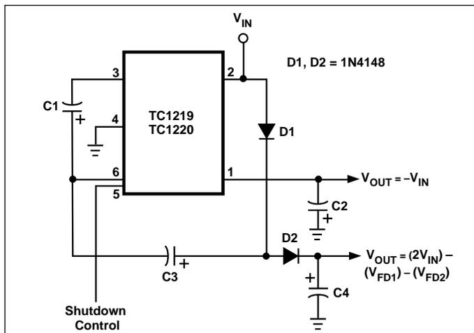
Figure 6. Combined Doubler and Inverter
