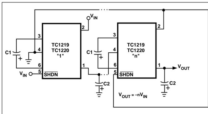
Figure 4. Cascading Multiple Devices to Increase Output Voltage
