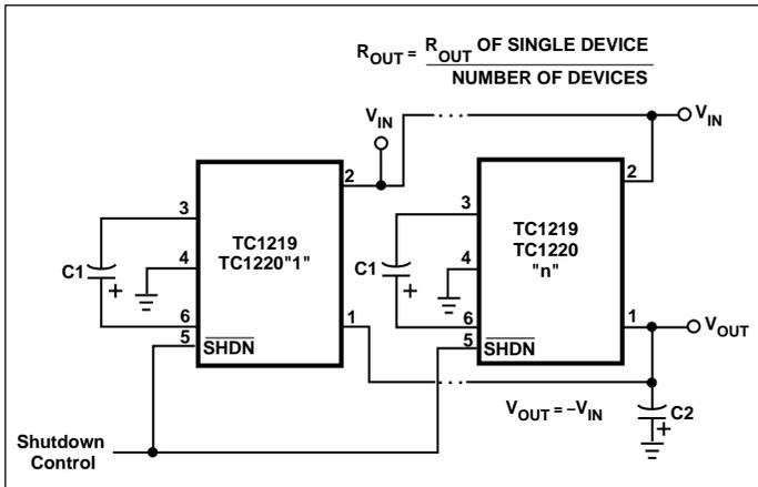
Figure 5. Paralleling Multiple Devices to Reduce Output Resistance
