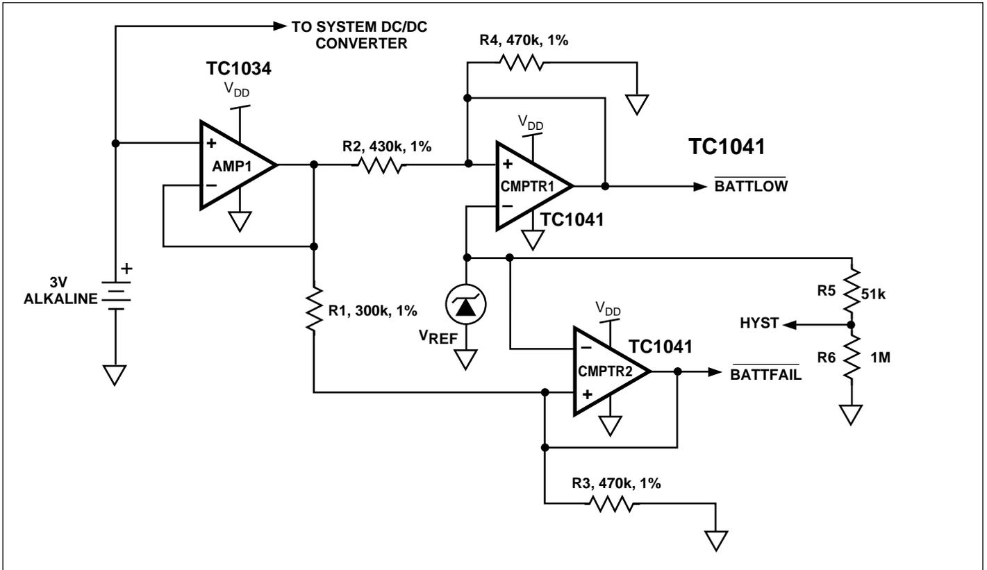
Figure 2. Precision Battery Monitor
