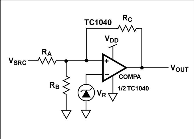
Figure 3. Comparator External Hysteresis Configuration
