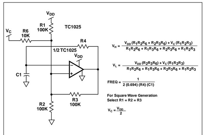
Figure 5. Pulse Width Modulator
