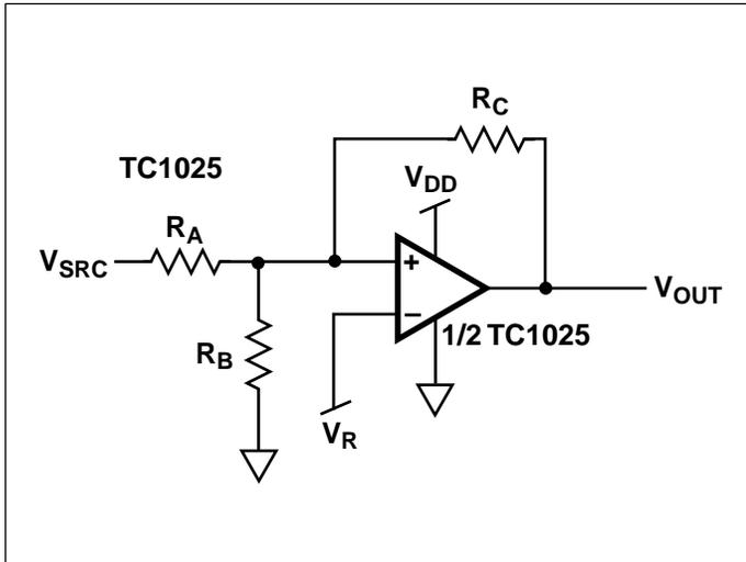
Figure 1. Comparator External Hysteresis Configuration
