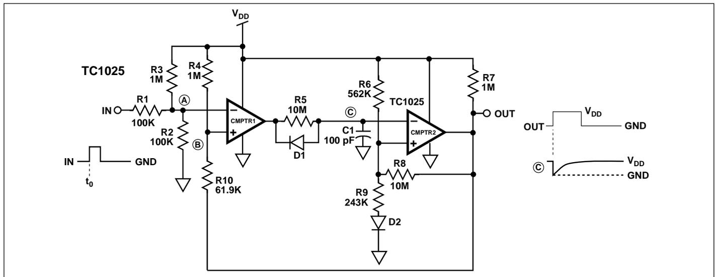
Figure 3. Non-Retriggerable Multivibrator
