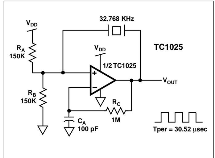
Figure 2. 32.768 KHz "Time of Day" Clock Oscillator
