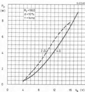
Fig. 2 - Maximum power dissipation vs. supply voltage (sine wave operation)
