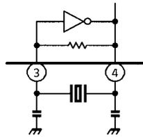
The start transfer frequency  $f_{st}$  and maximum transfer frequency  $f_{mx}$  depend upon crystal oscillation frequency  $f_x$ . Please make sure of the start operation in determining your frequency.
