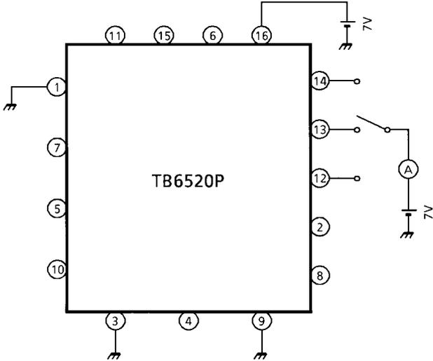
**TEST CIRCUIT 6:  $I_L$  (H)**
