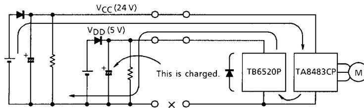
When the GND line goes open, the capacitor on the low-voltage power supply side is charged with a high voltage from the 24 V line through a circuit shown above. When GND is connected next time, the device may be broken by that voltage.
