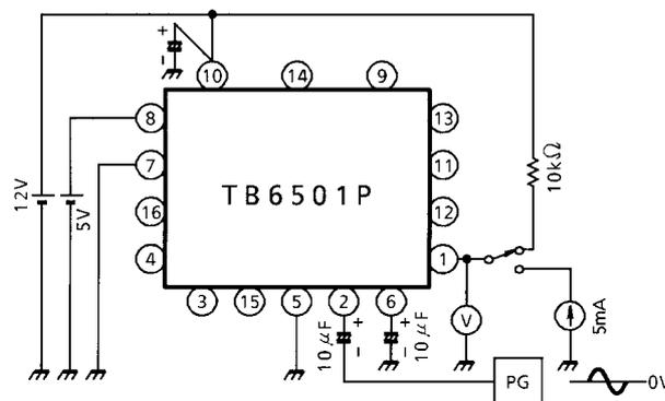
Note: Utmost care is necessary in the design of the output line,  $V_S$ ,  $V_{CC}$  and GND line since IC may be destroyed due to short-circuit between outputs, air contamination fault, or fault by improper grounding.
