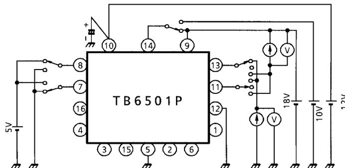
Note: Calibrate  $I_O$  to 0.2 / 0.4 / 1.0 A by  $R_L$ .
