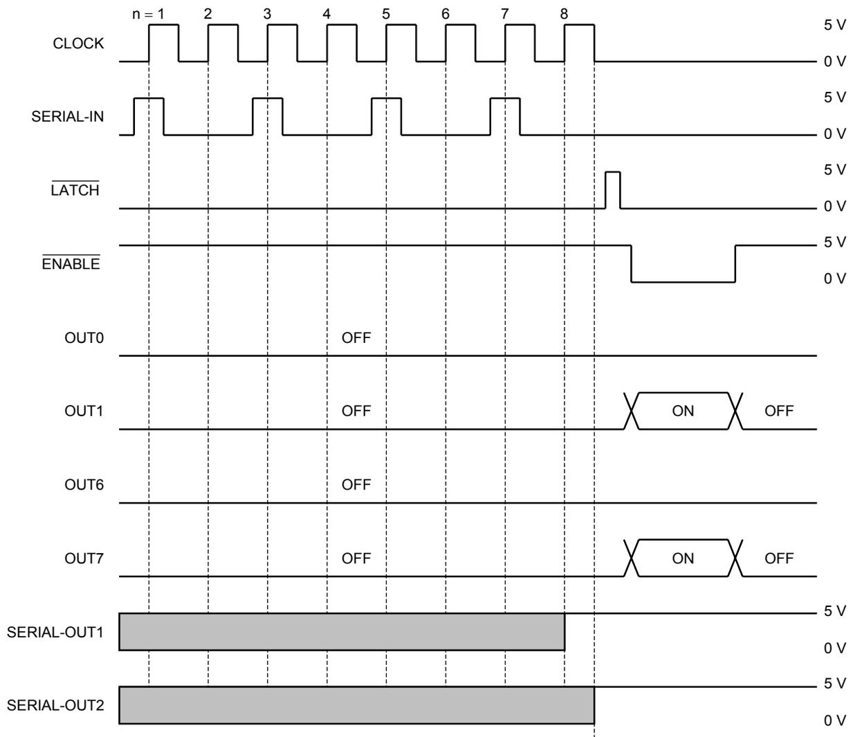
Note 2: The latches circuit holds data by pulling the  $\overline{\text{LATCH}}$  terminal Low.
