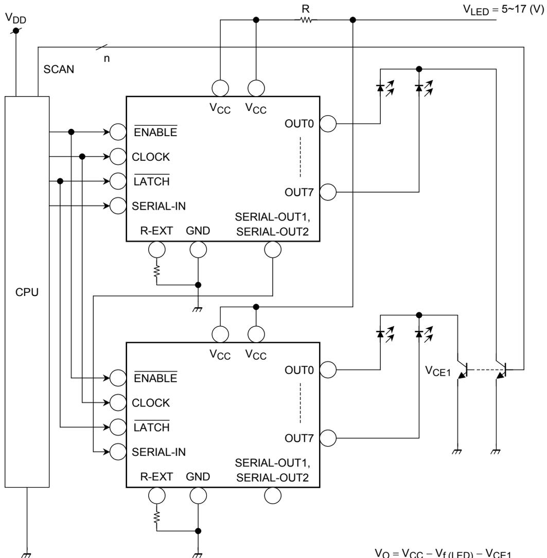
$$V_O = V_{CC} - V_f (\text{LED}) - V_{CE1}$$
