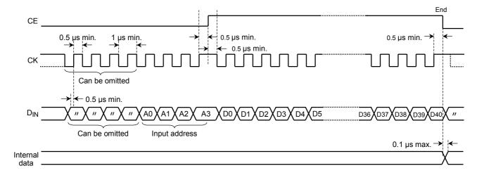
(Note) • When power for TB2118F is fully on, input data after 100ms or more.
