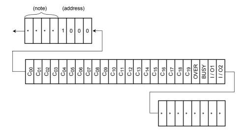
(Note) Either "0" or "1" can be set in bits marked with \*.
