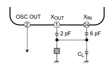
(Note) Use a crystal oscillator with  $R_S$  =  $50\Omega$  and less and  $C_L$  = 12pF or less.
