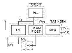
The above is an application circuit example of a 3-band (FM, MW and LW) 5-V tuner.
