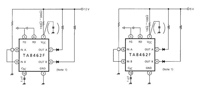
Note 1: In order to prevent the mutual induction of a motor, connect a additional diode between each output to motor. Note 2: Utmost care is necessary in the design of the output line, V<sub>CC</sub> and GND line since IC may be destroyed due to short-circuit between outputs, air contamination fault, or fault by improper grounding.
