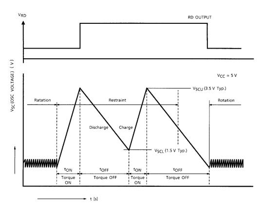
Fig.1 Auto mAtic Self Rotation Recovery Circuit Operation
