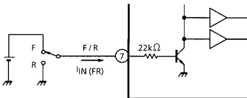
**2. Start / stand-by control input (RS input, pin (8))**
