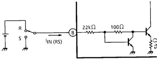
**3. Hall sensor inputs ( $H_a^{+,-}$ ,  $H_b^{+,-}$ ,  $H_c^{+,-}$ , pin (1), (2), (3), (4), (5), (6))**
