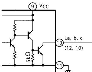
**5. Pre-drive stage (Ia, Ib, Ic, pin (16), (15), (14))**
