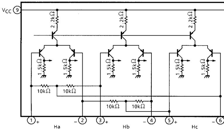
Wide DC operating range of  $0 \sim V_{CC} - 1.2 \text{ V}$  is accomplished by PNP input circuit and also built in hysteresis restricts mis-function caused by external noise.
