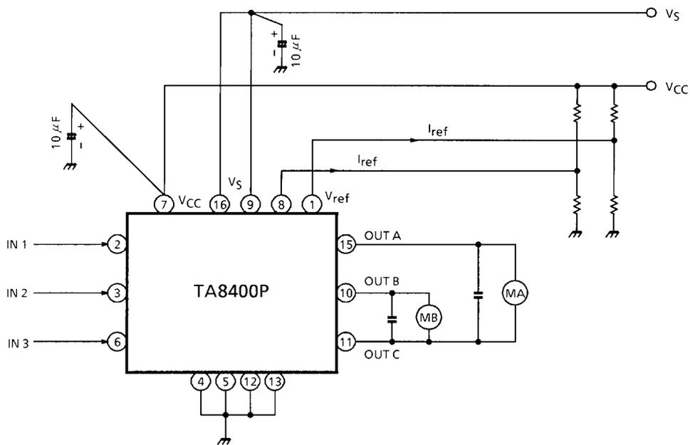
Pin (16) is required to connect to pin (9).
