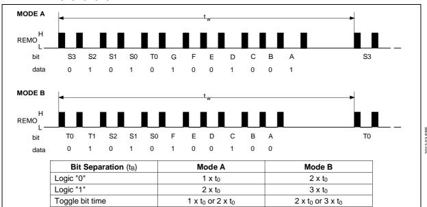
**Figure 1 :** Data Format of REMO ; T0 and T1 = toggle bits ; S0, S1, S2 and S3 = sub-system address ; A, B, C, D, E, F and G = command bits
