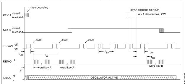
**Figure 4 :** Multiple Key-stroke Sequence. Scan rate multiple key-stroke :  $t_{SM} = 8$  to  $10 \times t_0$ .
